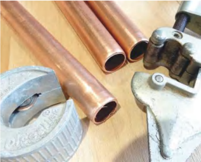
PIC 1. It worried me that the tube cutter rounded over the end of the pipe, which presumably would affect its clarity of tone. I tried being gentler with it, and I tried the cutter on the left but there wasn't much to choose between them. This does demonstrate, however, that if the bells were to be made of higher grade alloy, more attention would have to be paid to the method of cutting
